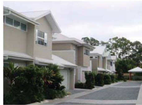
Parking integrated into the building design. Varied materials for access road punctuates and visually shortens the length of the access road. Change in materials can act as traffic calming.
