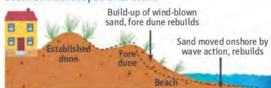
Figure 4. Natural short-term erosion and dune rebuilding process
