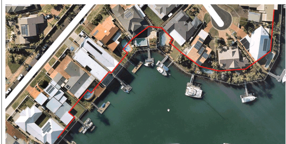
Figure 6.2.1.2.7 - To achieve compliance with PO8, dwellings may develop closer to the canal/lake, up to the red line. The centre of a site is used to delineate the location on the site where the red line changes to reflect the setback of the adjoining dwelling.
