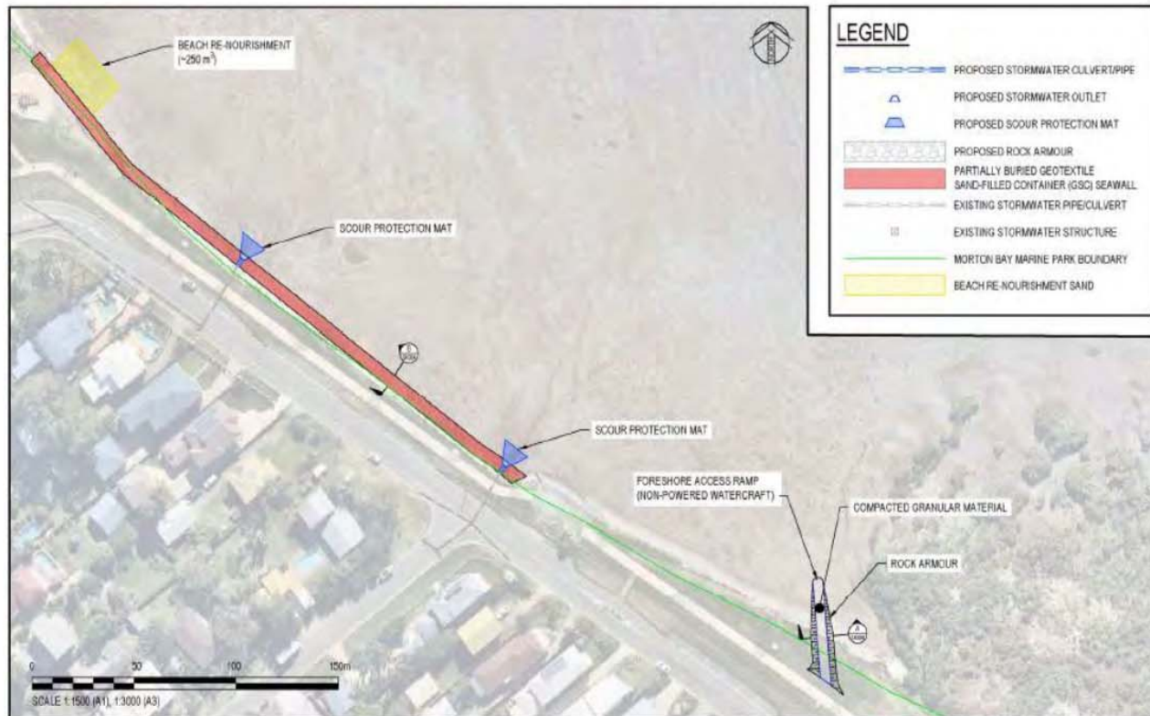
Figure 3.1 Proposed shoreline protection scheme, Queens Esplanade foreshore, Thorneside (Cardno 2019a).
