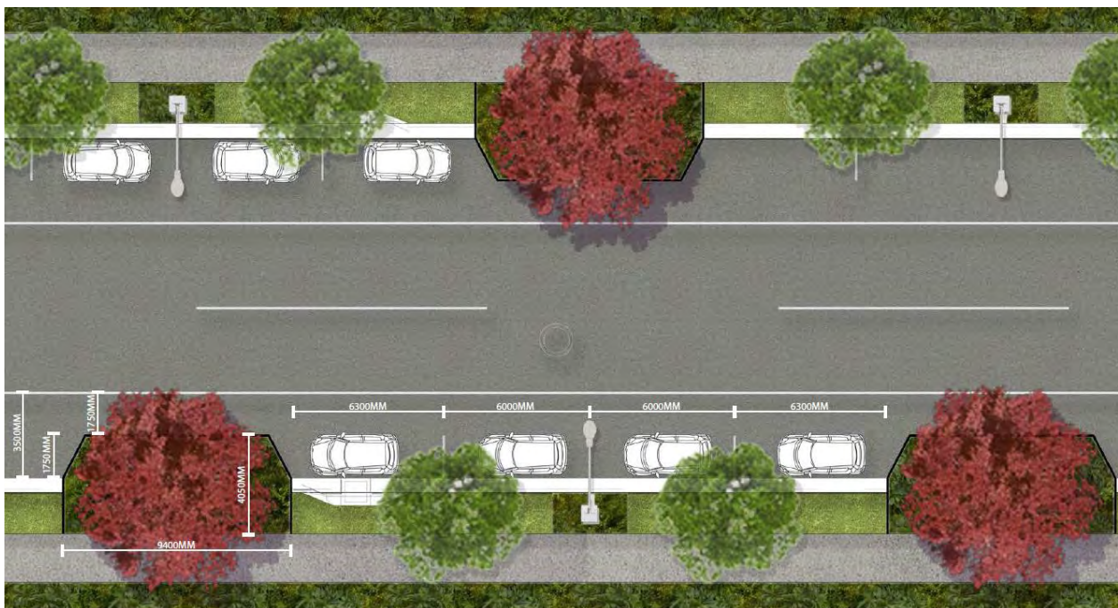
Figure 6: Tree build-outs on trunk collector
