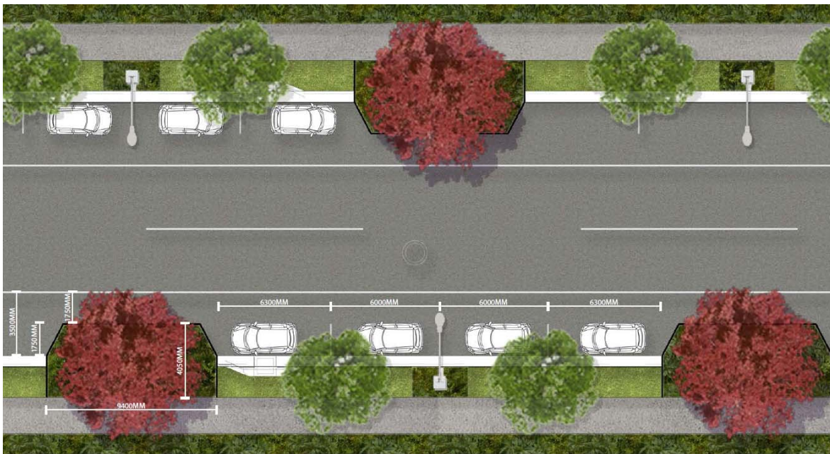
Figure 6: Tree build-outs on trunk collector
