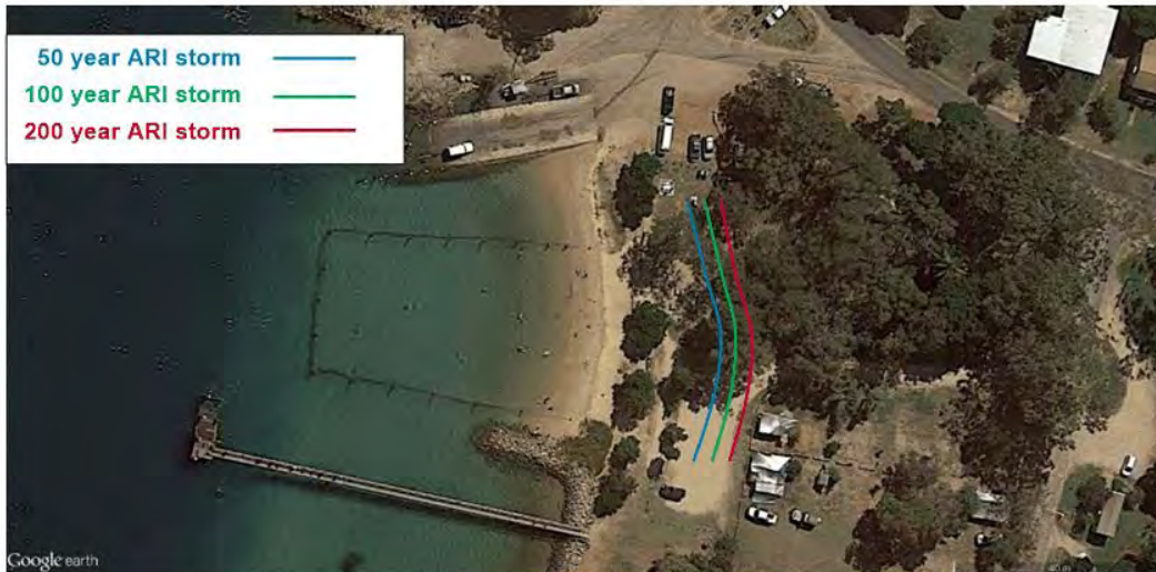
(a) Recession Lines on northern-most beach compartment – Southern Reach
