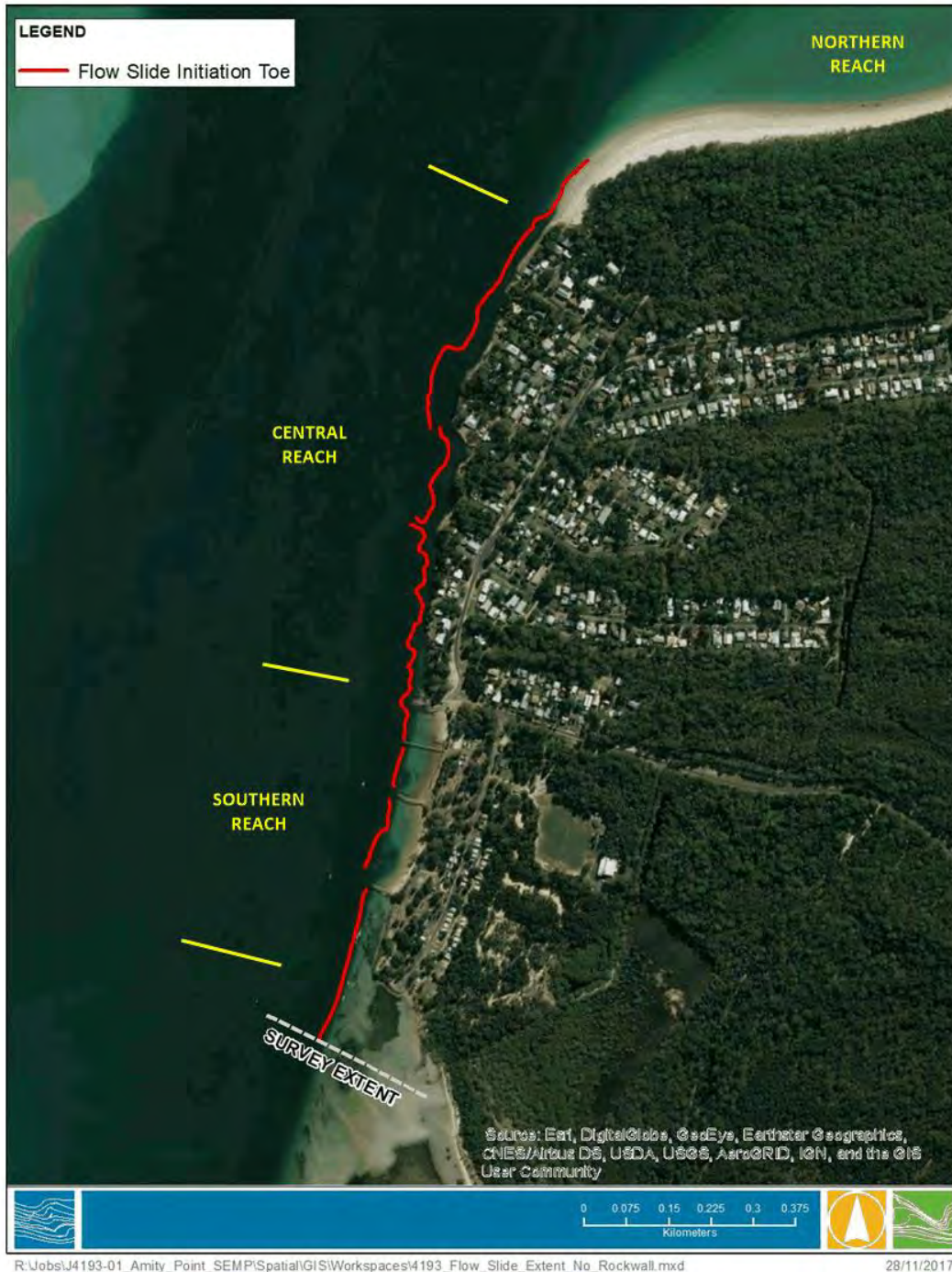
FIGURE 4-4 POTENTIAL LOCATIONS FOR INITIATION OF RETROGRESSIVE FLOW SLIDES
