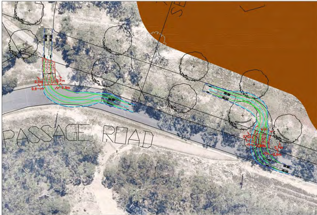
FIGURE 7.6- 12.5 METRE BUS MANOEUVRING
