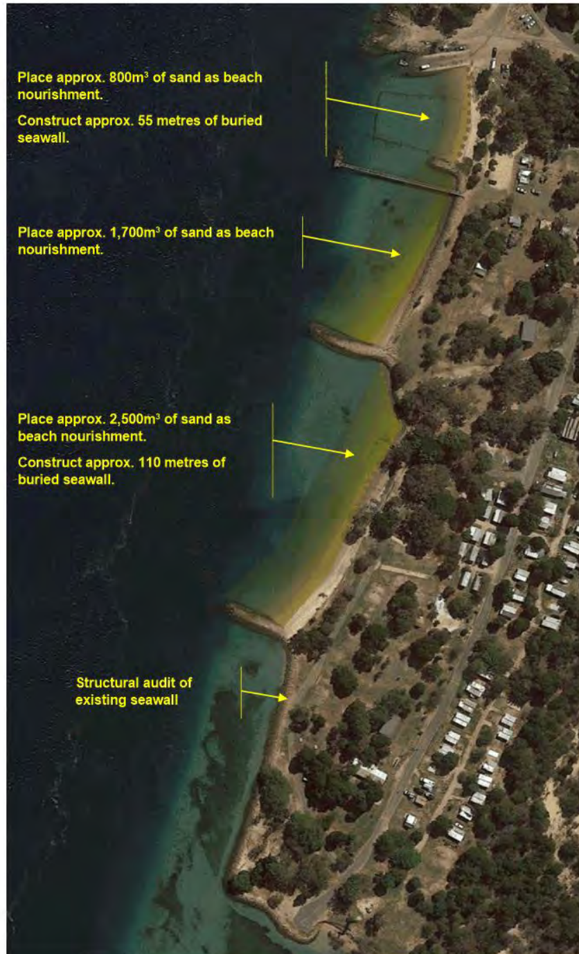
FIGURE 9-1 RECOMMENDED EROSION MITIGATION STRATEGY – SOUTHERN REACH
