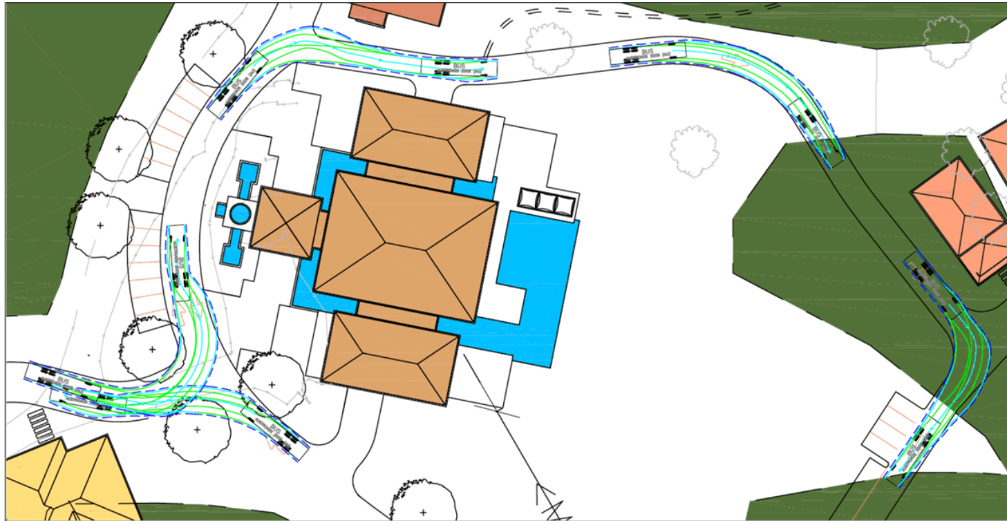
FIGURE 7.7- 12.5 METRE BUS MANOEUVRING
