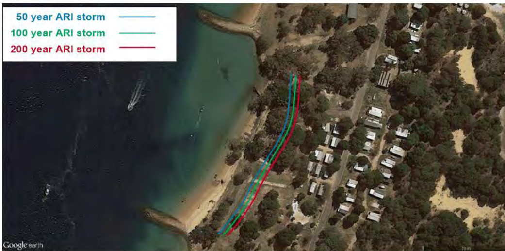
(b) Recession Lines on southern-most beach compartment – Southern Reach
