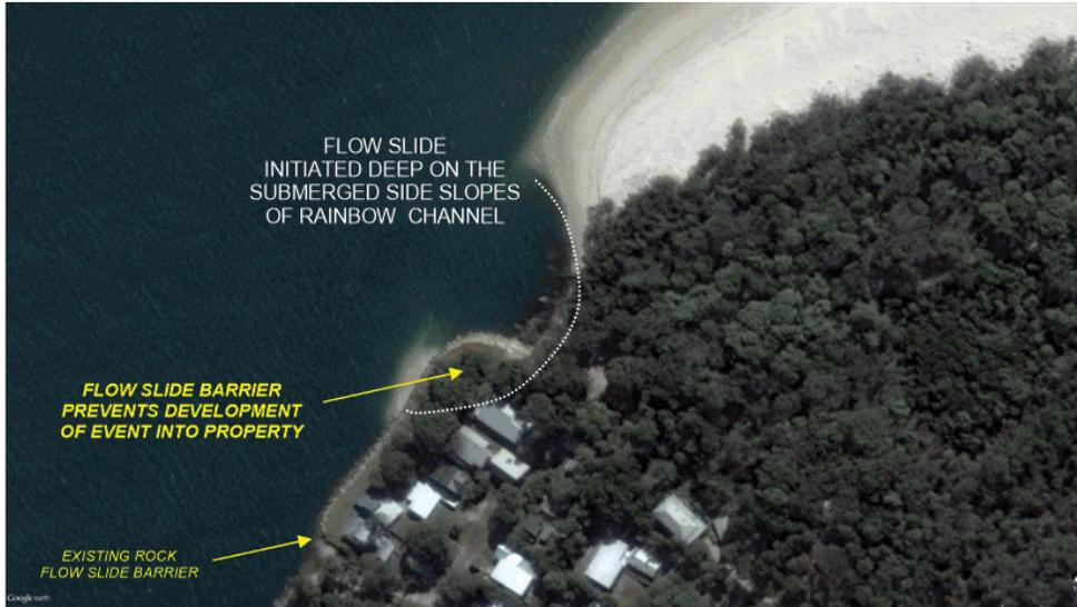
FIGURE 6-1 EXISTING FLOW SLIDE BARRIER INHIBITING DEVELOPMENT OF FLOW SLIDES
