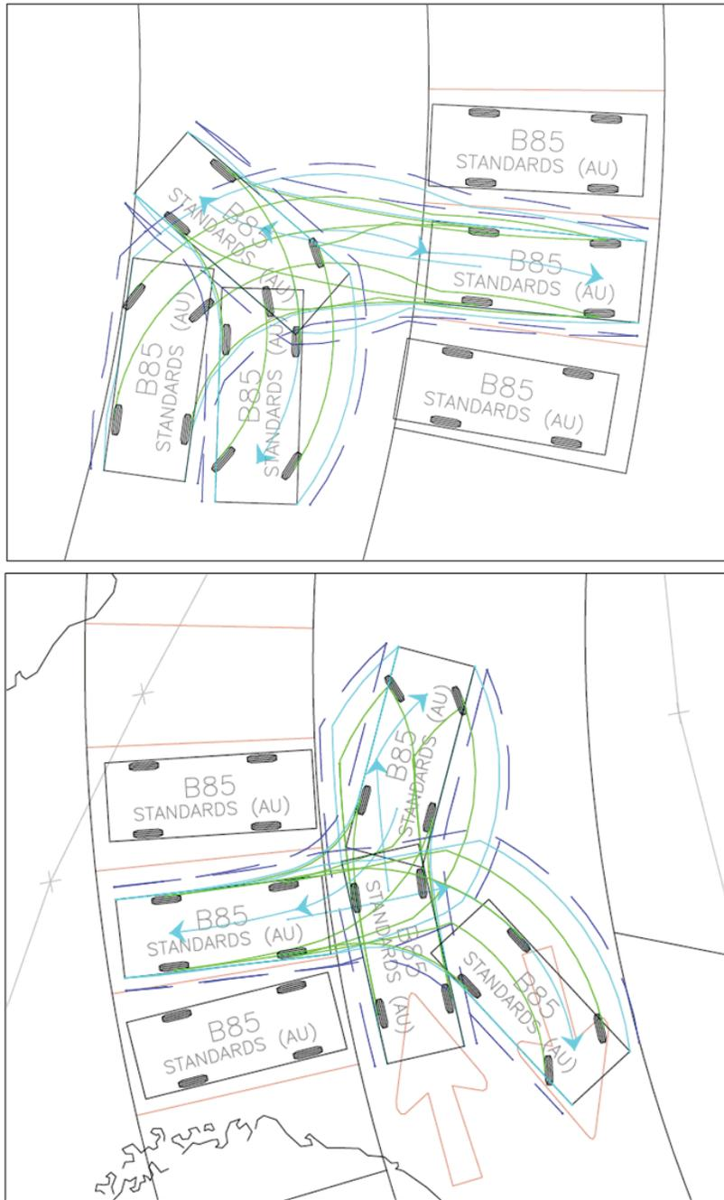
FIGURE 5.2 – 85<sup>TH</sup> PERCENTILE VEHICLE MANOEUVRING
