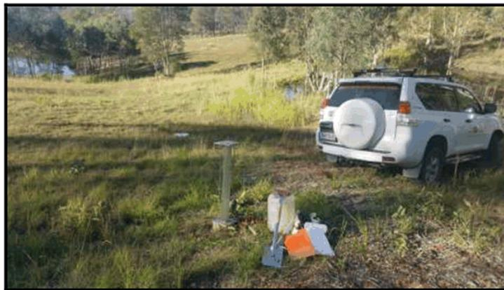
Figure 7: Typical setup of the field permeability testing facing north-east at the location of PT 8.
