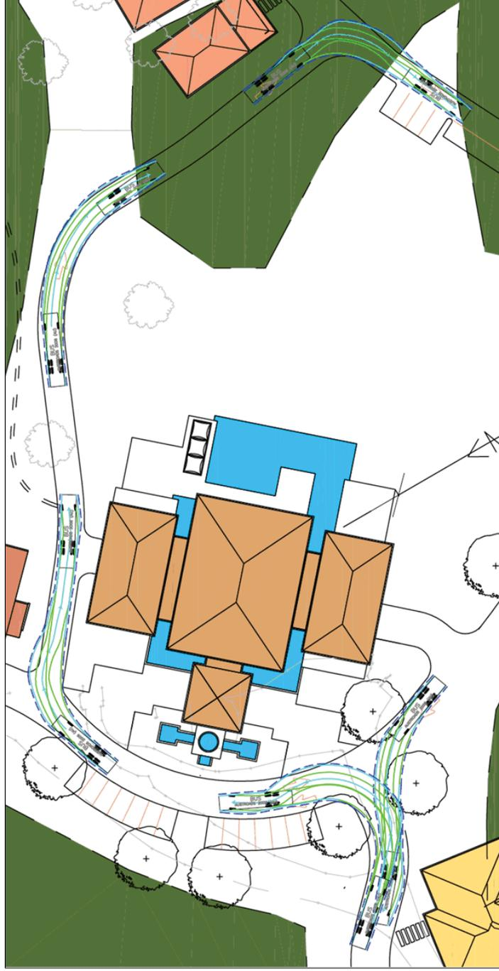
FIGURE 7.7 – 12.5 METRE BUS MANOEUVRING
