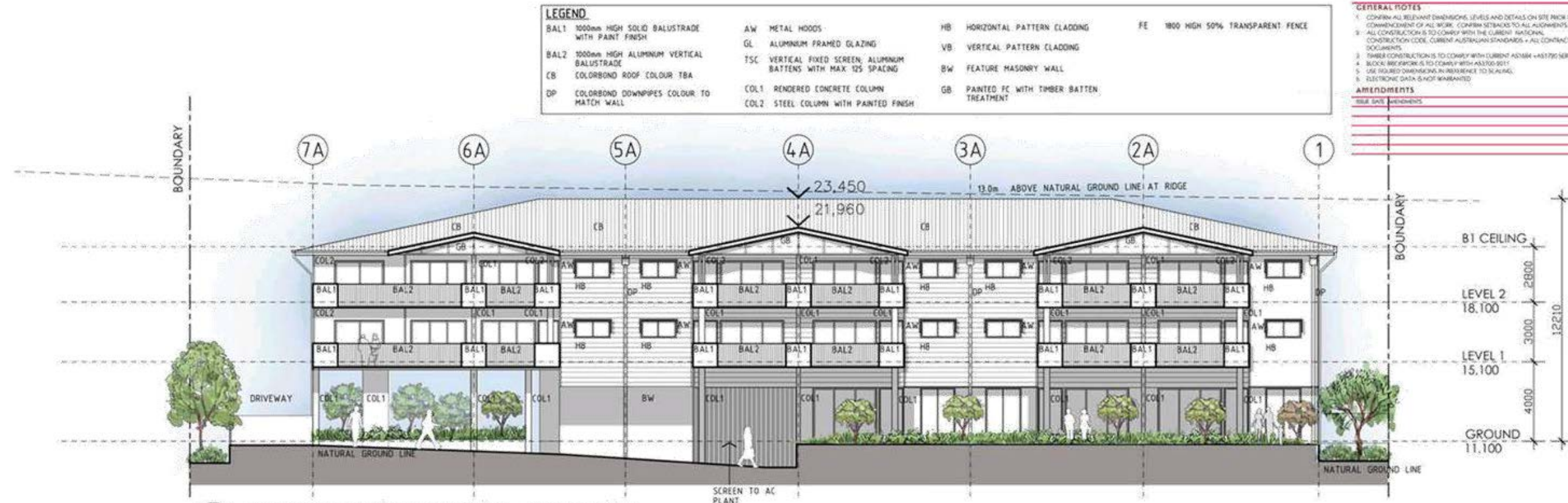
1 INTERNAL EAST ELEVATION - BUILDING 1 SCALE 1:200
