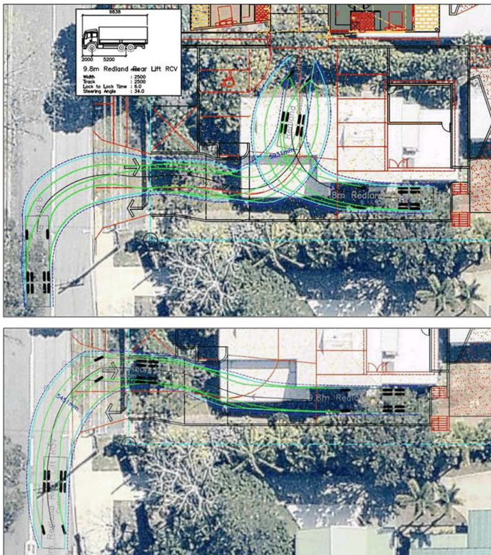
FIGURE 8.2 – 9.8 METRE REAR LIFT RCV MANOEUVRING
