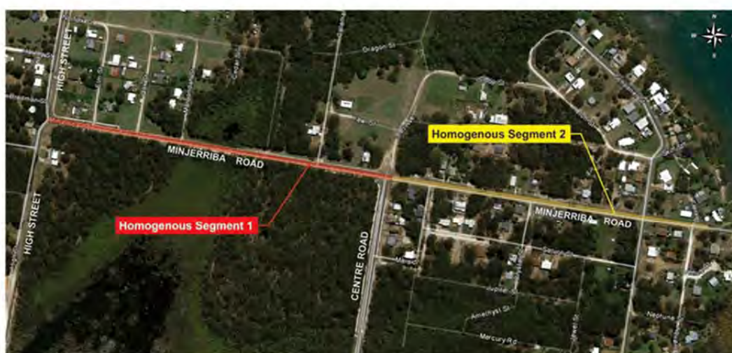
Figure 2: Homogenous road segments
