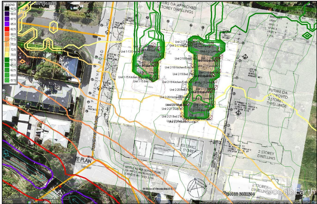
Plate B4: Noise contours, Level 4. Forecasts are in dB(A) L max , free-field
