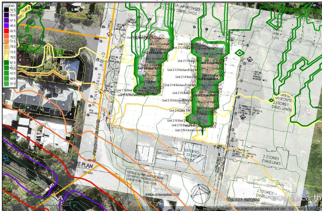
Plate B3: Noise contours, Level 3. Forecasts are in dB(A) L_{max} , free-field.
