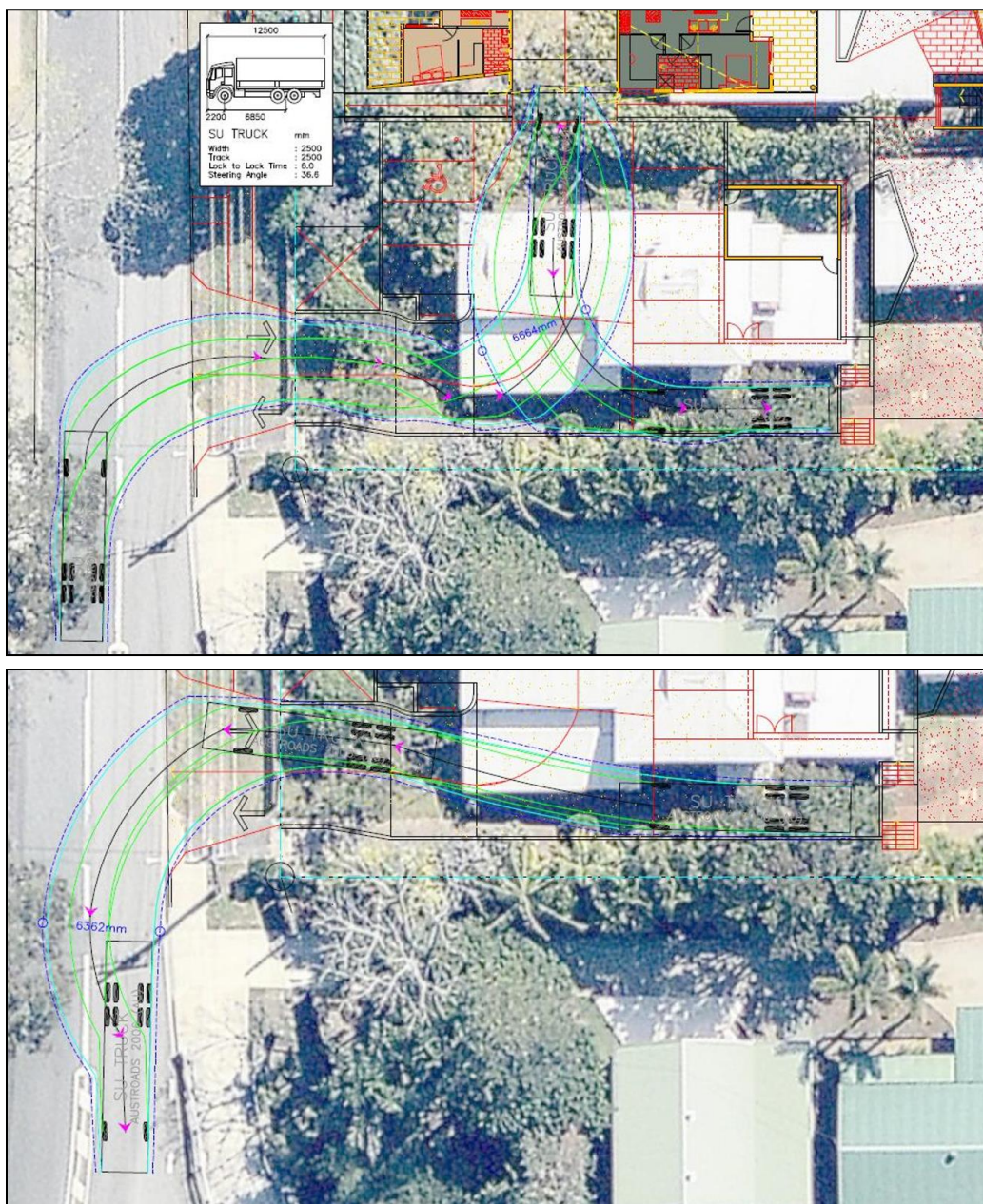
FIGURE 8.1 – 12.5 METRE HRV MANOEUVRING
