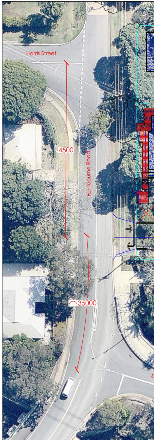
FIGURE 7.2 – DRIVEWAY PROXIMITY TO NEARBY INTERSECTION
