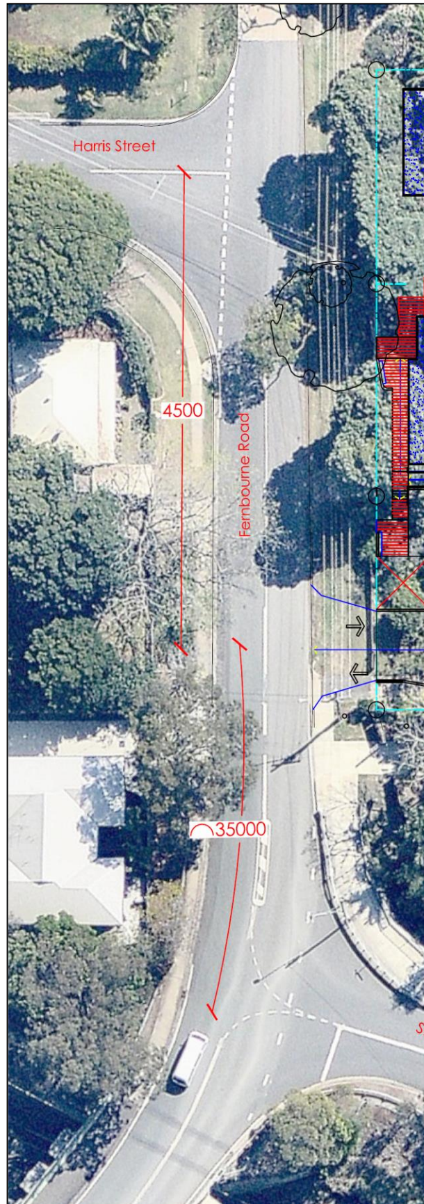
FIGURE 7.2 – DRIVEWAY PROXIMITY TO NEARBY INTERSECTION
