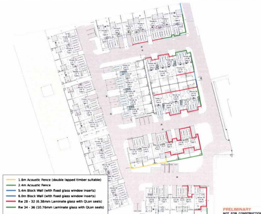
Figure 4 – Modelled Acoustic Barriers and Façade Treatments
