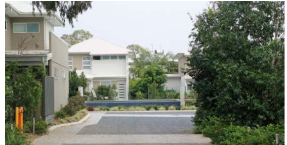
Figure 8 Entrance to site has a strong landscape setting. The varied paving materials throughout the site defines the shared surface and encourage a low speed traffic environment.
