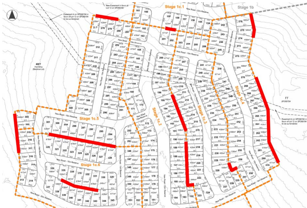
Figure 16 - Stage 1c retaining walls over 1.5m in height
