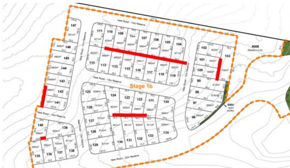
Figure 15 - Stage 1b retaining walls over 1.5m in height
