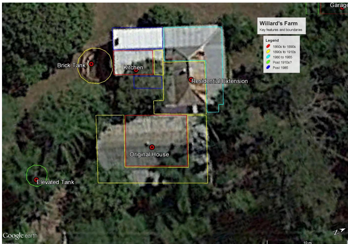
Figure 10: Stages of construction of the residential complex – core of original residence and elements of kitchen (c.1860s - red); brick tank, residential extension and southern verandah/walkway with skillion roof, later additions to kitchen including pantry and stairs (c.1890s to 1910s - yellow); verandahs to north and west of residential extension and western extension (c. 1980 to 1984 -light blue); verandah to west of kitchen and roof over kitchen stairs (post 1985 - dark blue).
