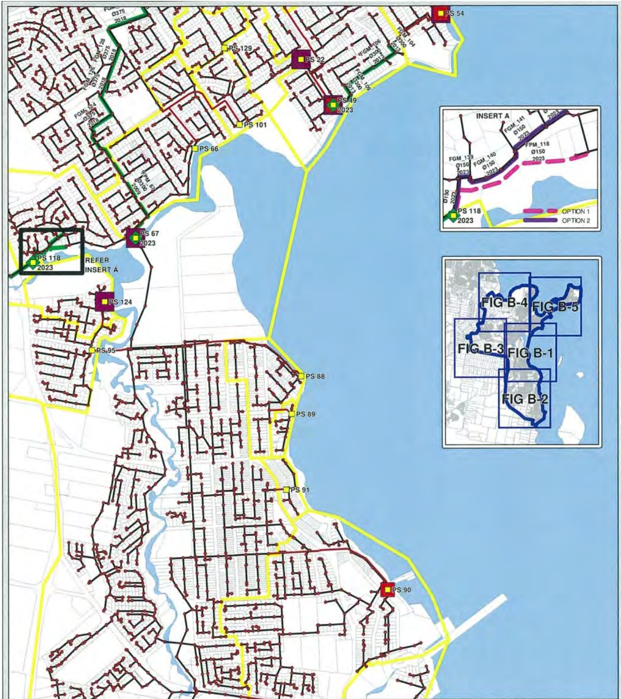
FIGURE 6 – TYPICAL REDLAND CITY COUNCIL SEWERAGE NETWORK
