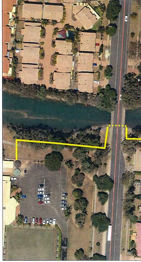
Middle Street Pipe Crossing (Underneath Road)
