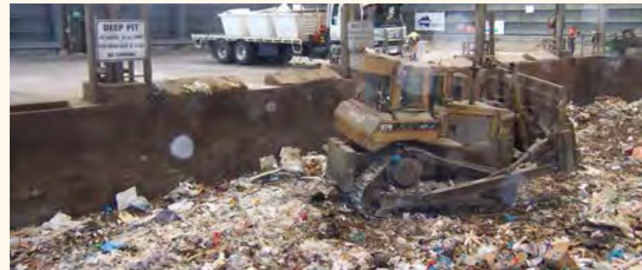
Examples of transfer station push pits
