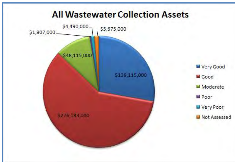
GRAPH 5. WASTEWATER COLLECTION CONDITION
