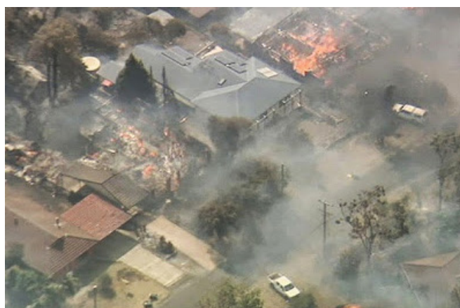
ABC News photograph of buildings that have succumbed to ember attack from the Blue Mountains, NSW fires in 2014. The unburnt condition of the vegetation around the buildings is evidence of ember attack on unprotected and probably undefended buildings.
